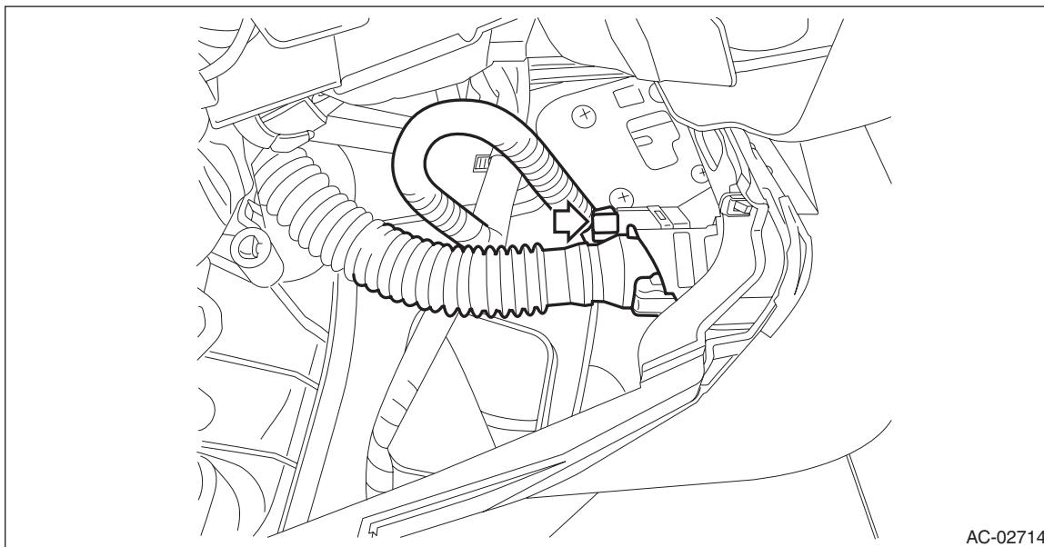
(2) Release the claws, and then remove the panel - switch.
